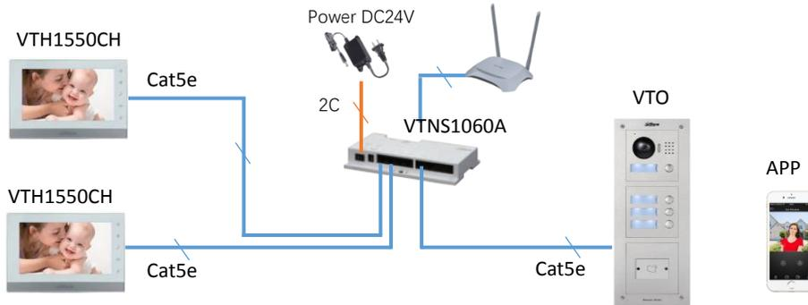
**Note:** VTH1550CH and VTO can be powered by VTNS1060A. Moreover, these devices can be powered individually with 12V/1A if you use other IP switch. **Maximum support for 40 flat.**
