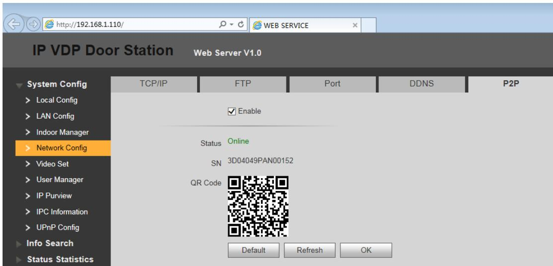
Step 3 Open the 'DMSS' App -> 'Door', touch '+' to add new device. Select 'P2P' connection way to connect with VTO2000A.
