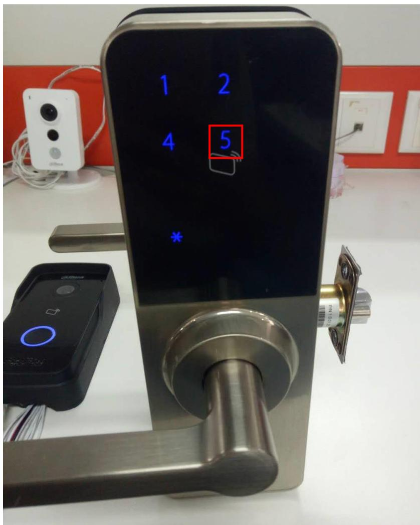
Step 4 Press the call button for 5 seconds. There will be three beep, representing VTO are In connecting mode. Wait a few seconds. If it comes **one beep**, it represents successful connection. If there is three, try again from step 2.
