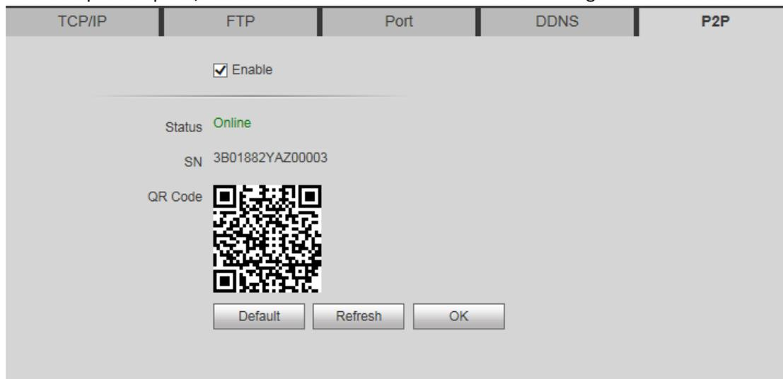
Step 4 Add device on smart phone. Enter add device interface. Press P2P. Enter name, scan QR code at rear of the device or you can also input S/N manually, press Start Preview finally.
